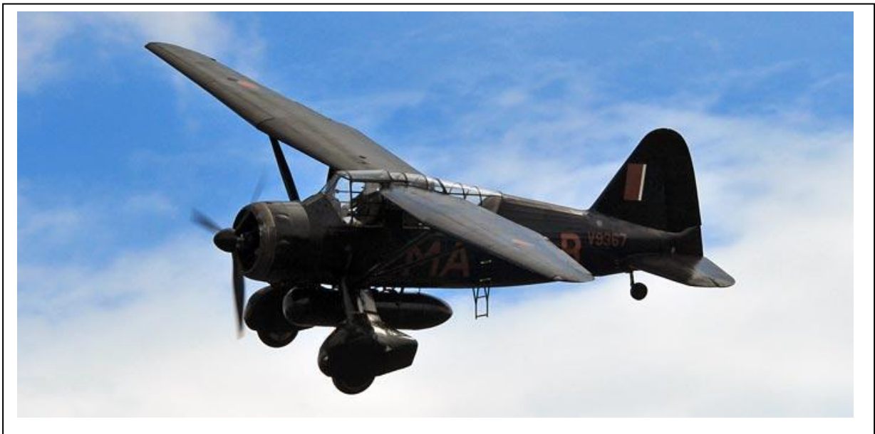
The fixed ladder shown here was put there to get agents in and out as fast as possible.
